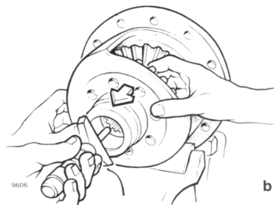
Differential gear shim thickness (16, page 7).
