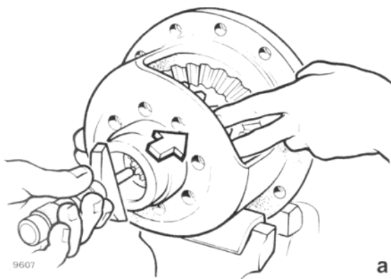
Differential gear shim thickness (16, page 7).
