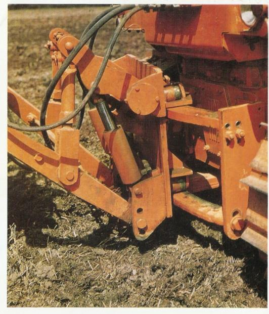
While the tractor is under heavy pull load, the linkage swings off centre, allowing the tractor to run on the unploughed land without steering interference.
