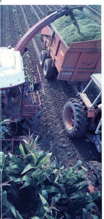
The ground drive transmission is fully hydrostatic. Elimination of the gearbox makes it possible to reduce power take-off and transmission consumption.
