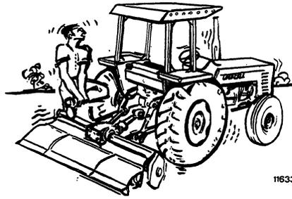
■ Before attempting to inspect, clean, adjust, repair or service the tractor or coupled implement in any way, ensure that the engine is shut off, transmission in neutral, brakes are applied, PTO is disengaged and all moving parts are stationary.
