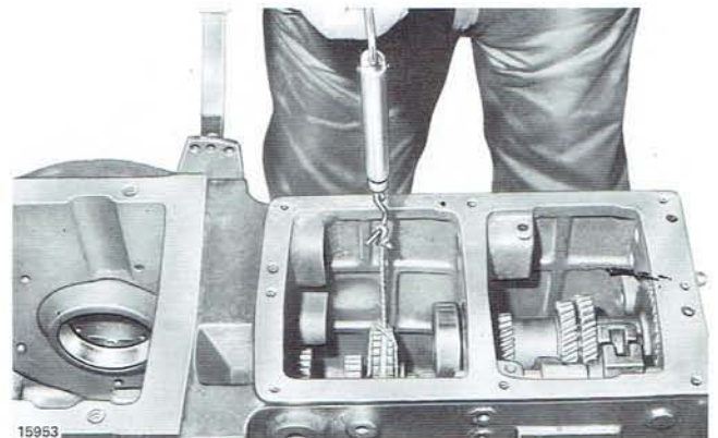
Bevel pinion taper roller bearing adjustment.
