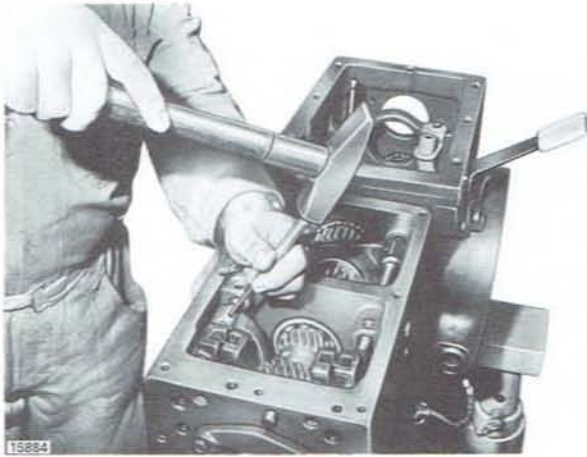
Removal of resilient pins securing transmission/splitter shifter fork and detent plungers.
