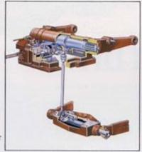
Two auxiliary rams are provided as standard on the 130/140/160/180-90. These result in high maximum liftable loads on the 160/180-90 tractors up to 7420 kg.
