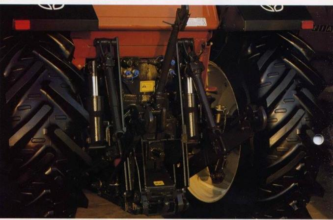
With draft, position and mixed control. The draft control operates through an oilbath flexion bar housed inside a separate assembly mounted under the rear part of the transmission. The hydraulic system is an original Fiat design and monitors the operation of the implement under all conditions, even under varying loads and soil resistance.
