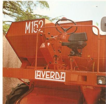
The operator's platform is in the best position to view the whole cutting platform.
