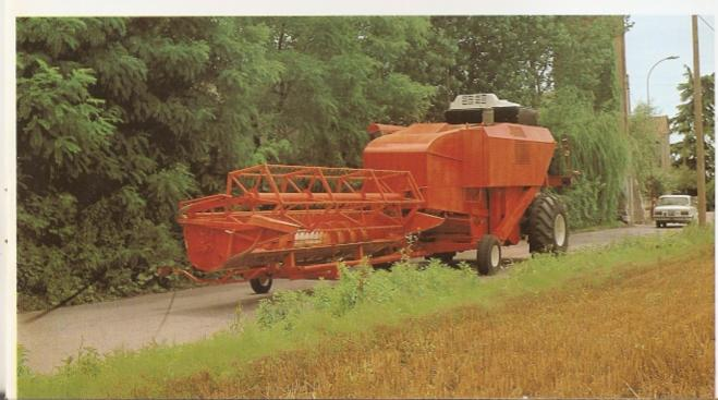
The cutting table is of new design. The knife drice has the wobble box in in oil bath, the knife runs at high speed and the ball joint has automatic adjustment of the backlash.
